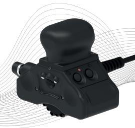
SG NDT WAVE probes are specially designed to perform handheld inspections of carbon steel and stainless-steel welds that have a rough surface finish. The probe is equipped with dynamic lift-off technology, which makes it ideal for inspecting painted welds without having to remove the paint. The probe's memory stores calibration data, making it easy to use and access when needed.
